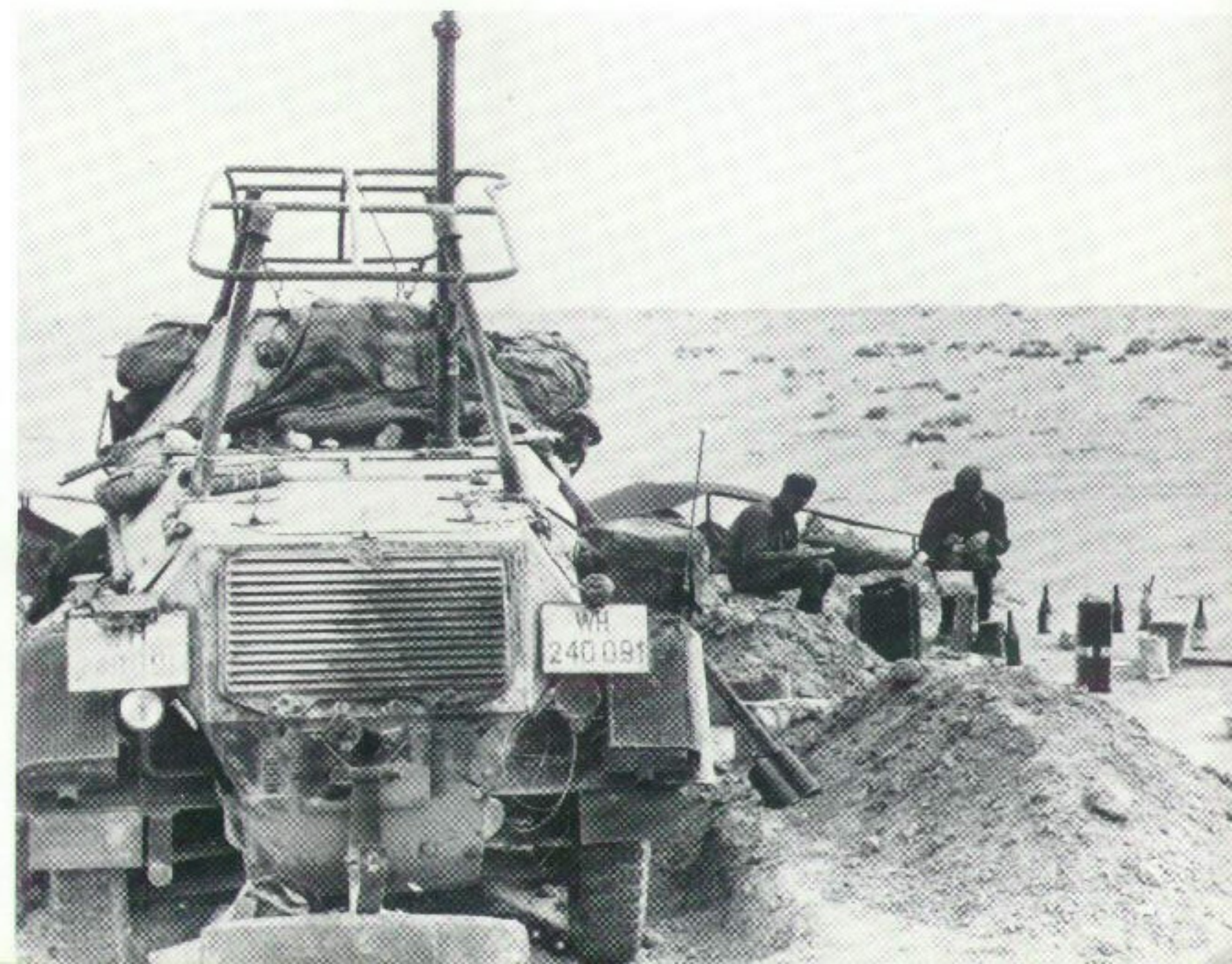
This SdKfz 263 of PzRgt 5, 5th leichte Division, has been camouflaged with a slurry of mud. Note the vehicle is parked in a shallow pit. This was intended to lower the silhouette somewhat and also to protect the tires. Often during midday, cloth covers were stretched over the wheels to shield them from direct sunlight. Like most other vehicles in the desert, this radio car has a good deal of extra crew stowage. [Bundesarchiv]
