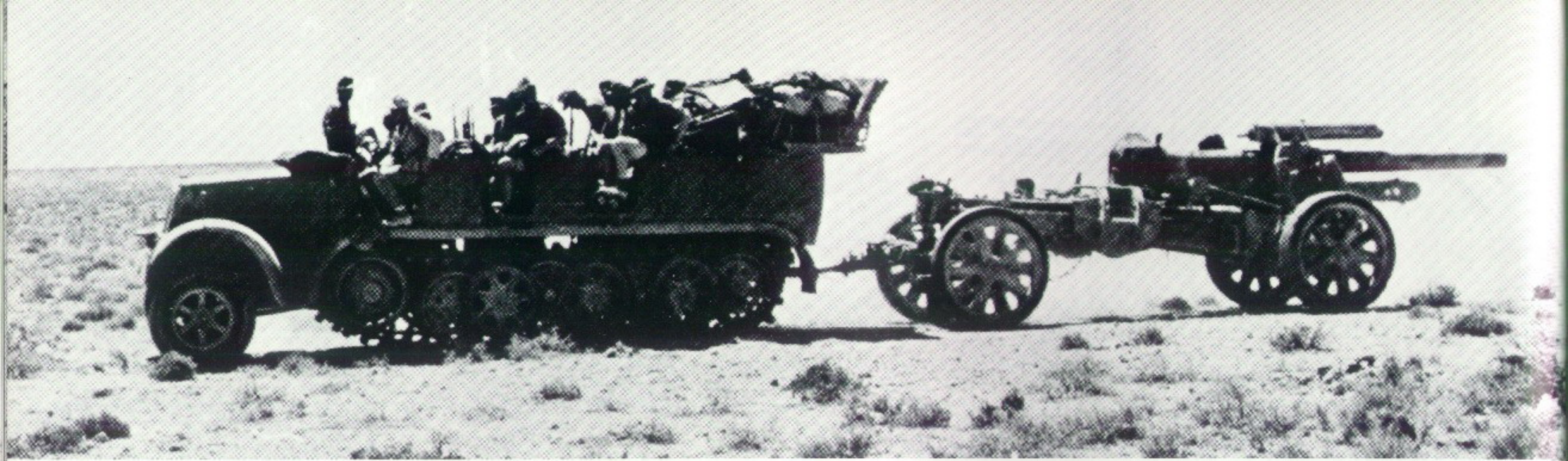
The 15 cm sFH 18 was the standard German medium field gun. Here, one is being towed by an SdKfz 7 tractor near Gazala in April 1942. For long distances, the barrel was disconnected from the recuperator system and carried in full recoil position to shorten the gun and make it easier to negotiate sharp corners in built up areas. [Bundesarchiv]
