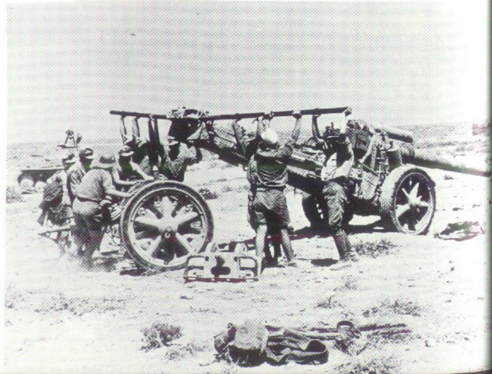
One step in the emplacement of a 15cm sFH 18. Here, the trails are lifted off the limber which is then rolled to the side. Next the trail spades will be fitted and the piece will be placed in its prepared position for firing. Note the variety of uniforms found in this crew. Several alternative uniform combinations were possible. [Bundesarchiv]
