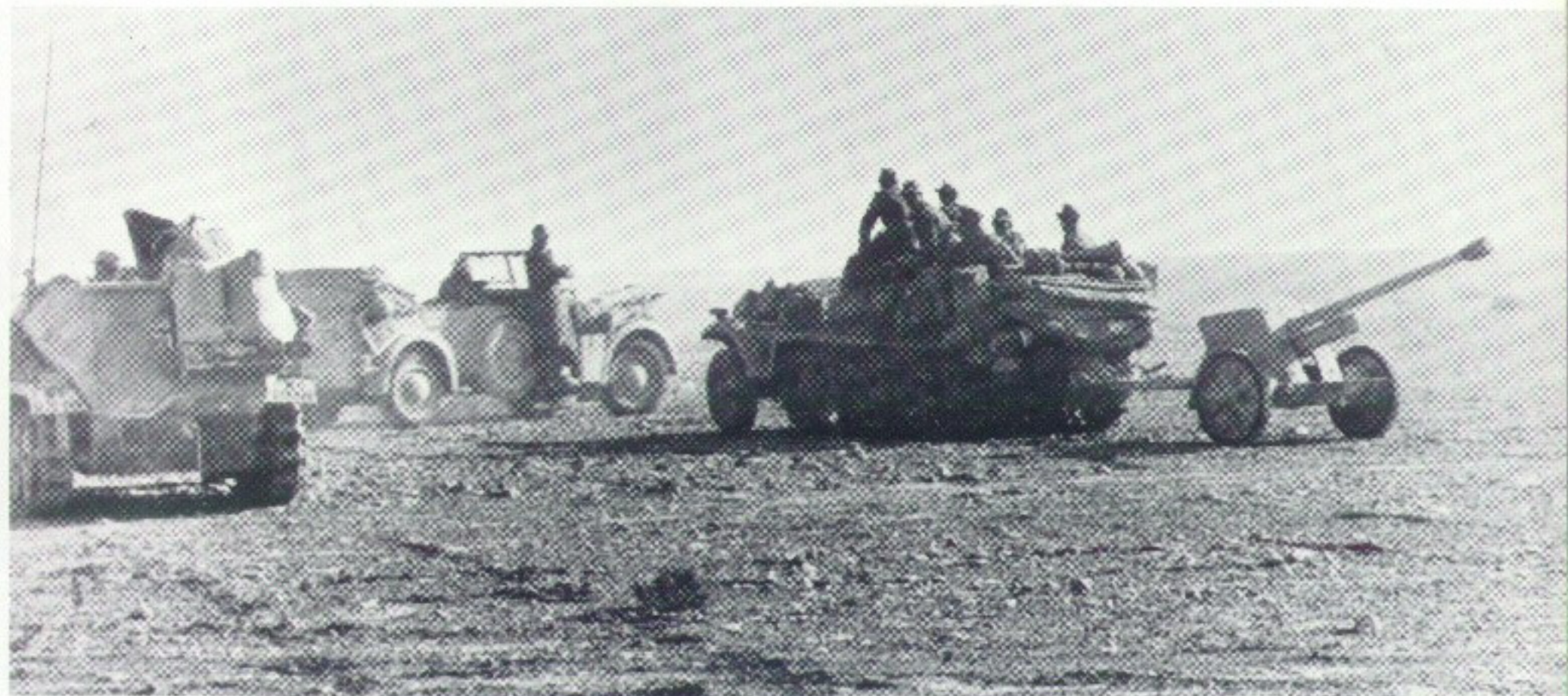
This SdKfz 232 [8 rad] armored car shows some of the modifications made by DAK personnel to make their vehicles more suitable for desert use. Extra tires have been piled on the engine deck and strap steel frames fabricated to hold 20 litre jerrycans of water. Many parts of the Western Desert had a good deal of sharp stones below the sand surface, and this combined with heat and mines, made provision of extra spare tires a wise move. [Bundesarchiv]
