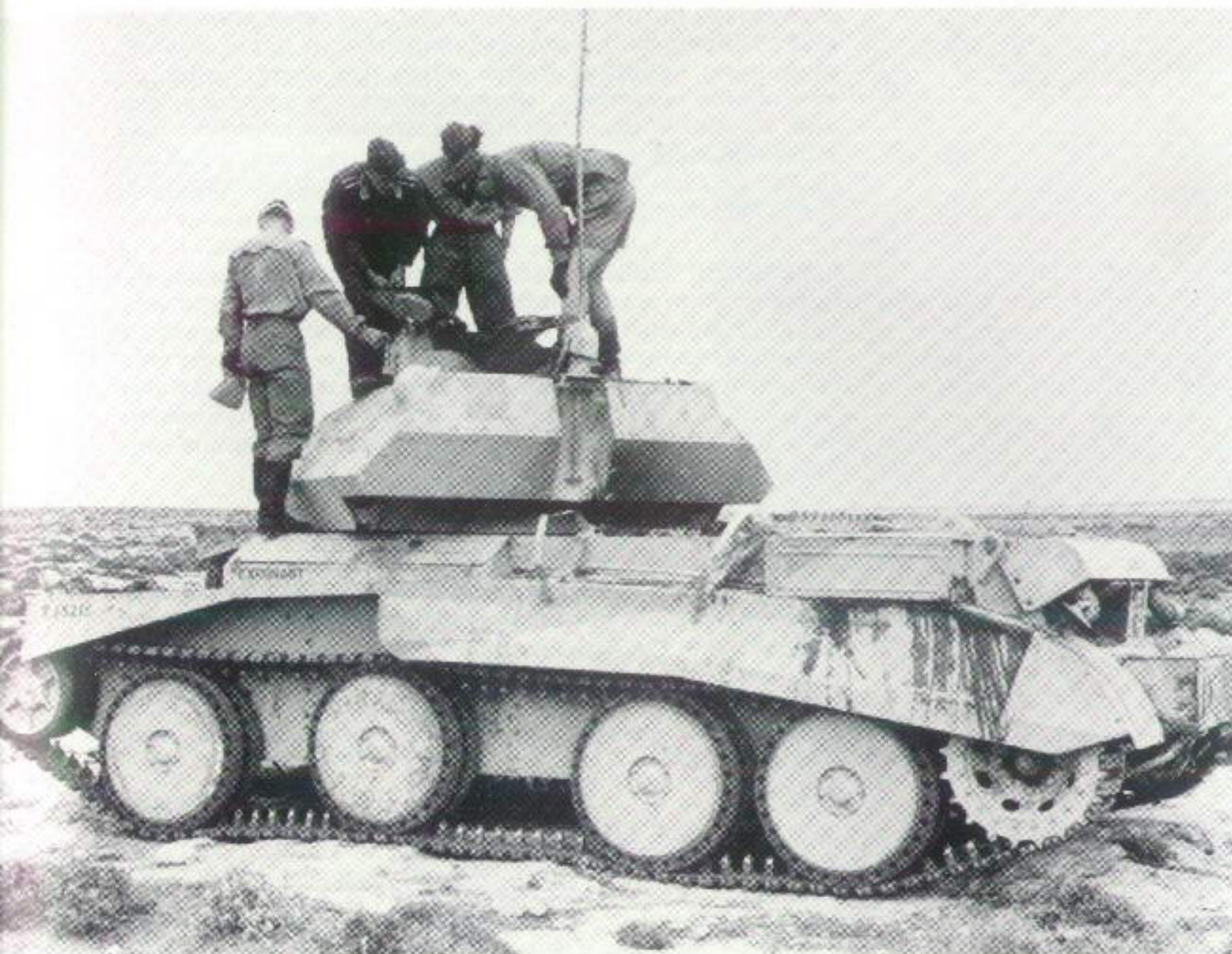
Several DAK soldiers examine a British A13 Cruiser tank, destroyed in an early engagement in 1941. Many early British tanks were plagued with various mechanical difficulties and their relatively thin armor could be penetrated at very long ranges by the 8.8 cm gun. [Bundesarchiv]
