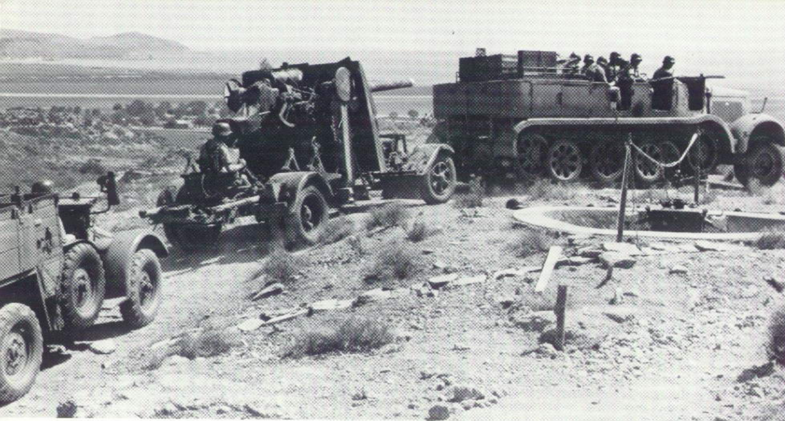
The 8.8cm Flak 18, seen here behind a SdKfz 8 12-tonne tractor, was Rommel's "secret weapon" in the early stages of the African campaign. Designed as a dual-purpose weapon for both anti-aircraft and ground targets, it proved to be the finest antitank weapon of the African campaign. General Rommel used these guns to destroy British armor at long range after using his own armor to draw out the enemy tanks. Following the Flak 18 is a Krupp Kfz 69 "Protze" light truck. [Bundesarchiv]
