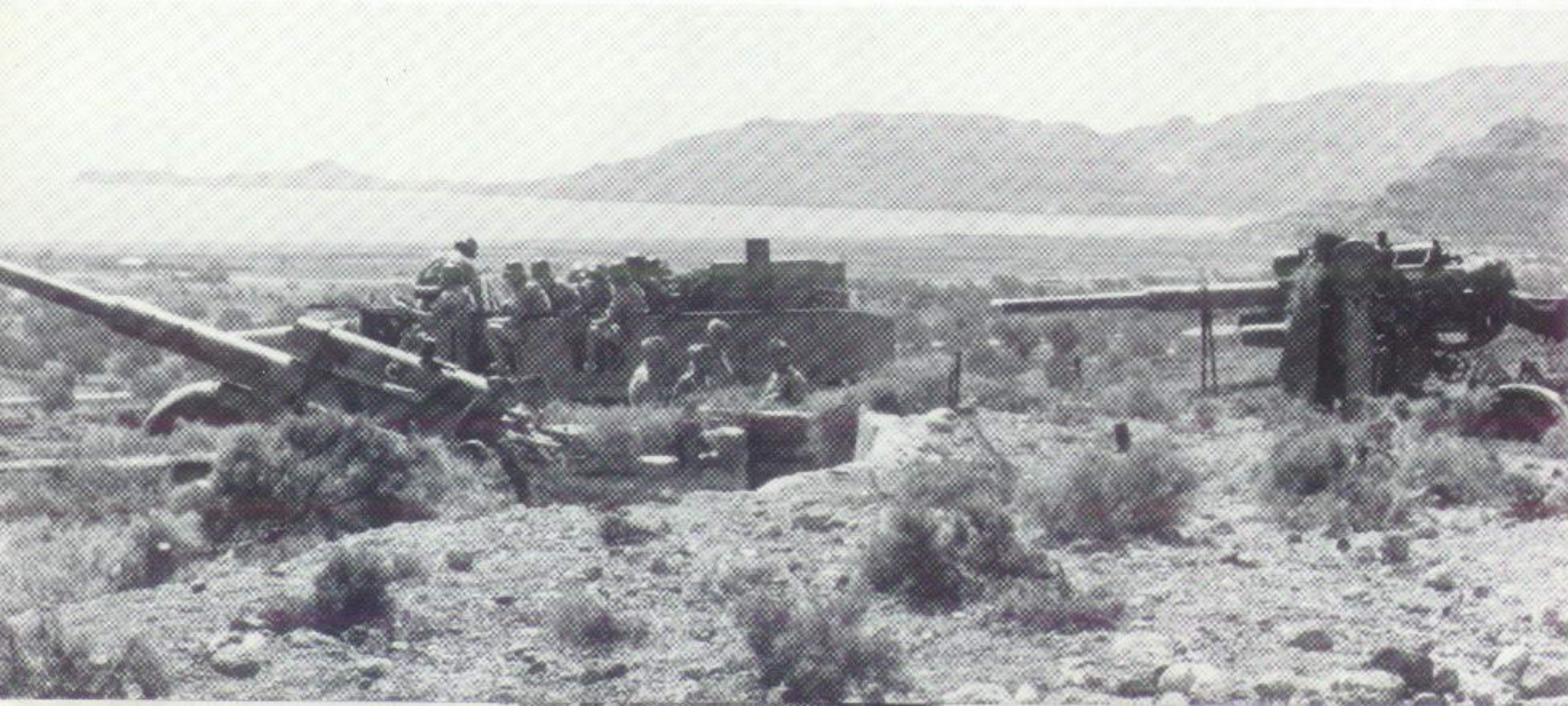
At the left, an 8.8cm Flak 36 of an antitank battery covers a section of coastal road in Libya as a second gun is towed past to its own position. Most "88s" were fired from prepared positions which allowed the guns to be set as low as possible, and afforded a measure of protection for the crews from counterbattery fire. The only major difference between the Flak 18 and Flak 36 was the barrel construction, the Flak 36 having a 3-piece liner which was easier to replace when necessary. [Bundesarchiv]
